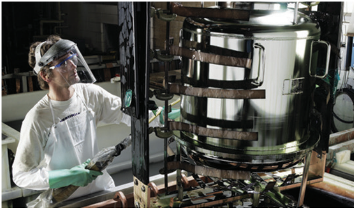
A portable vessel used in the pharmaceutical manufacturing industry emerges from the electropolishing tank at Apache Stainless Equipment Corporation.
